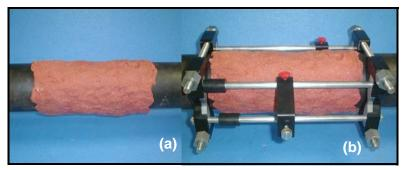
Figure 3-31: Spreading the DMP-3 (a) and Reinstalling the Fixture (b)
